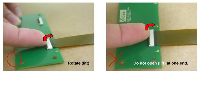
The actuator opens by rotating it in the direction OPPOSITE to the direction of the insertion of the FPC. DO NOT attempt to open it from the same side as the insertion of the FPC.
