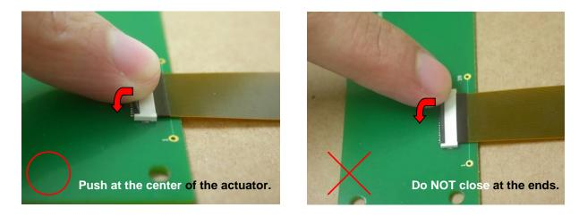
About the lock operation When you lock, it is recommended what the actuator does as a whole, and the actuator was shut surely.
